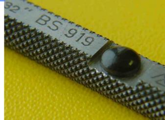
RFID system ilD $^{\$}$ 2000 closed coupling, 13.56 MHz, based on ISO 15693
